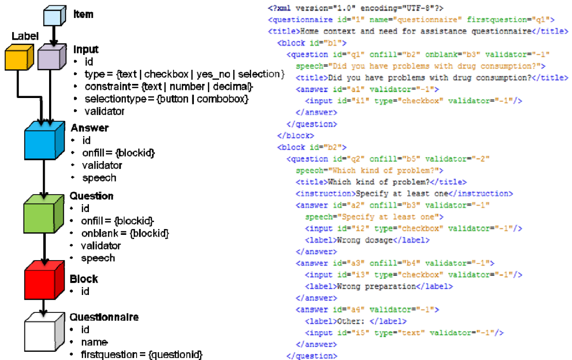
Figure 2. The XML elements representing the questionnaire on the left and an excerpt on the right. The excerpt refers to the questionnaire for the parents of preterm newborns.
